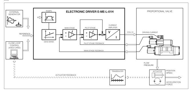
E-ME-L drivers control the current to the solenoid of Atos proportional valves with position transducer, regulating the spool position or the flow according to the electronic reference signal, adjusted by transducers's feedbacks.
